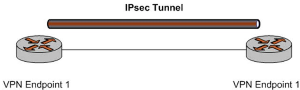
For site-to-site IPsec tunnels, the Brocade vRouter supports a special kind of interface—a virtual tunnel interface—that provides a routable interface at the endpoints of the tunnel.
