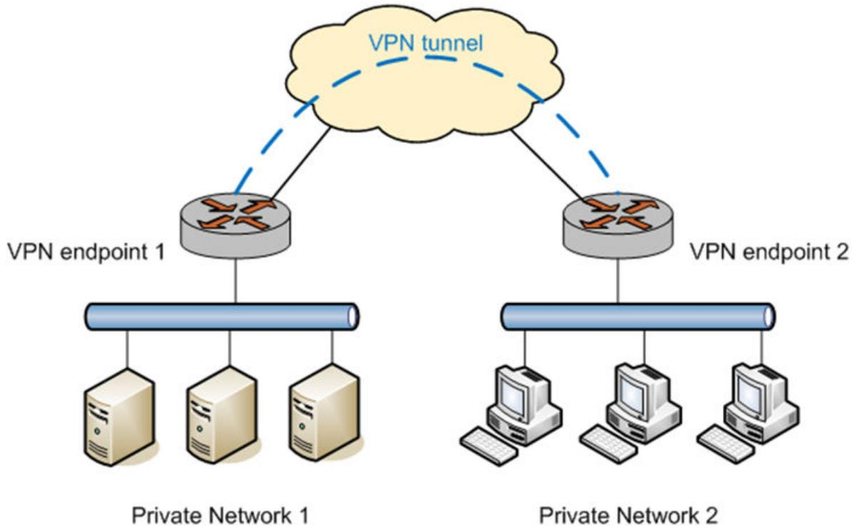
The following figure shows how the Brocade vRouter supports IPsec-protected site-to-site tunnels.
