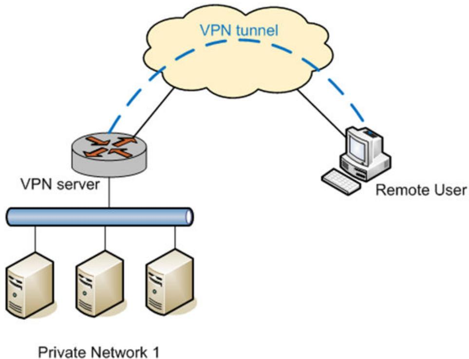
The following figure shows the one way option to implement a remote access VPN is by using Layer 2 Tunneling Protocol (L2TP) and IPsec.
